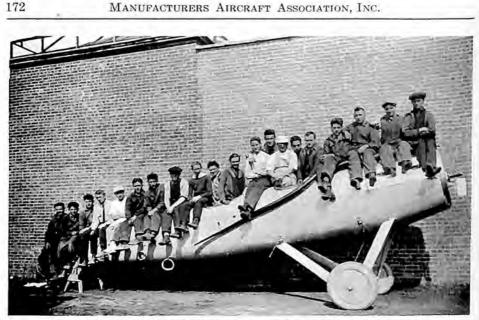
An L-W-F Fuselage for Model V. Note the twenty men which the shell supports
