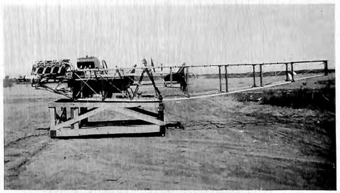
Secondary Fuselage Assembly, Aeromarine Model 39-B.
