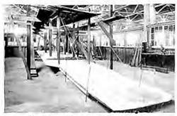
Sand Load Test of H-12-A Panels
