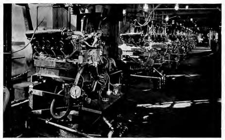
Testing the Finished Motors
