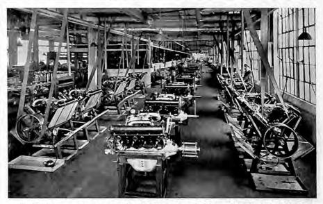
Finished Motors being Belted in. This is the finishing end of Assembling, the start of which is shown on page 276
