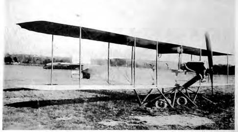
Burgess Tractor, showing first enclosed fuselage in United States
