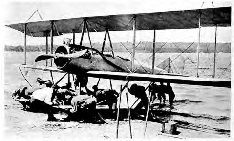
The first L-W-F Machine, equipped with Pontoons
