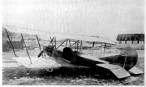
A later development of the Tractor Side-by-Side Seating Arrangement
