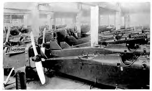
Group of De Haviland-4 fusclages ready for final assembly of wings, center sections, and tail surfaces
